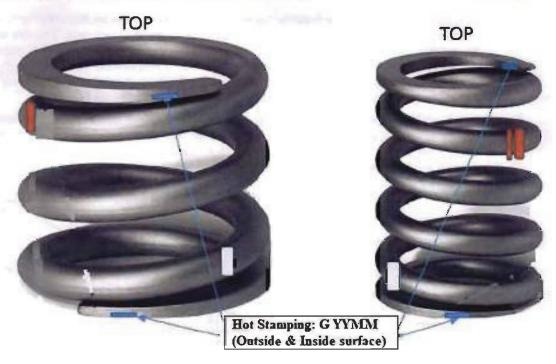
The material code shall be legibly hot stamped on both tapered ends of each spring in such a way that the particulars are visible on the outer surface of the ineffective coils and they do not get erased during end grinding or interfere with the performance of the spring. For drawing codes of springs Annexure-I may be referred.
