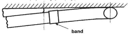
Further, the direction of free transverse deflection "ri" of every flexi-coil spring (category 'B') is to be marked with a band of aluminum adhesive tape (e.g. Tesaflex 171). The band is to be attached to the painted spring as in the sketch below:
